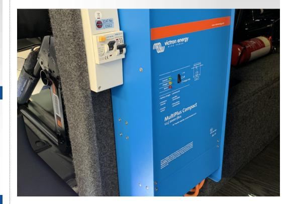
The inverter is located behind the front cab passenger seats in the rear saloon. Make sure that the black switch is set to 'ON' and the green light is showing. If the red light begins to flash it means that the battery is running low therefore the ignition will need to be turned on in order to recharge the battery.
