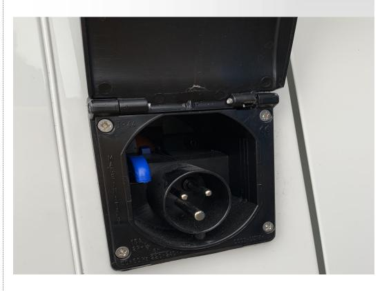
The external hook up can be found on the drivers side of the vehicle. This can be used to power the equipment on board instead of running on the vehicles battery.
